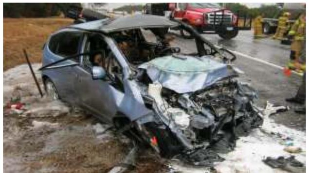
The court found that the improper repair procedures compromised the structural integrity of the vehicle and in the subsequent loss, the collision energy of the impact was not properly channeled away from the occupants as designed by the OEM manufacturer.
